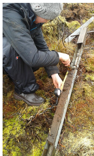
Figure 59 A box corer is simple to use: the front has been removed to show the sample © Andreas Heinemeyer
