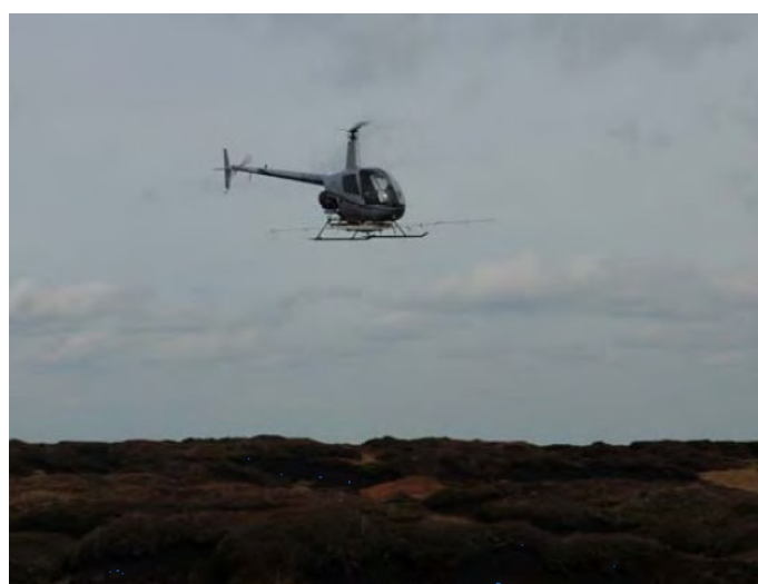
Figure 142 Helicopter hydroseeding © Moors for the Future Partnership
